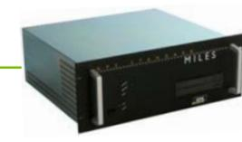
Thanks to the use of electronic/software filters the fence version of Miles™ analyses both the low and high frequencies typical of a climbing or cutting attack on the fence.
