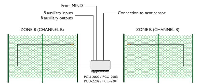
The sensor provides a series of NC contacts, via terminal blocks, for the signals of Pre-alarm, Alarm, Cut and Short for channel "A" and channel "B" and, in addition, the Fault and Tamper signals. The device can be programmed through the USB port or COMI I5 serial port. The length of the sensitive zones for both the version with 2 or 4 zones is 300m each. This distance is given by the sum of the insensitive cable (RG59) and the sensitive one used to protect the specific section of perimeter.
