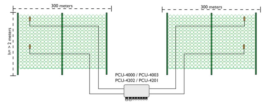
If the sections to be protected were sequential, the length of the two outer sections may be up of 150m since the beginning of the distant sections will be connected to the analyzer through a non sensitive cable with a length equal to those of the two sections closest to the analyzer:
