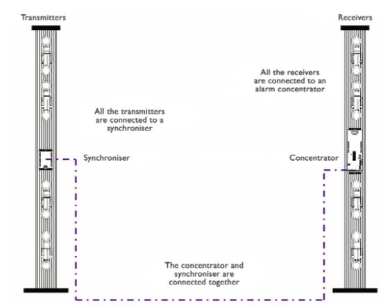
Many concentrators can be connected to universal communications processor (MIND) using a BUS cable for data and power.
